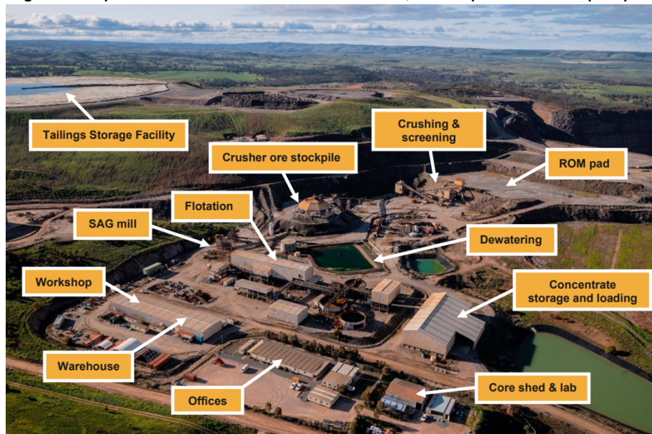
Figure 23: Layout of Kanmantoo's surface infrastructure, with ample additional capacity should mining rates improve or exploration succeed
